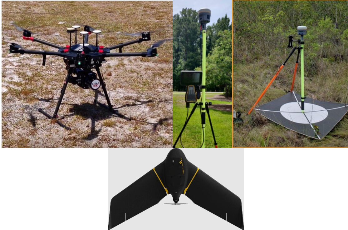
Figure 8. Images of platforms used for data collection. (Left) DJI Matrice 600 Pro with Quanergy M8 LiDAR sensor, (Middle) Trimble RTK R8 and R10, (Right) fixed wing eBee with parrot sequoia multispectral sensor.
